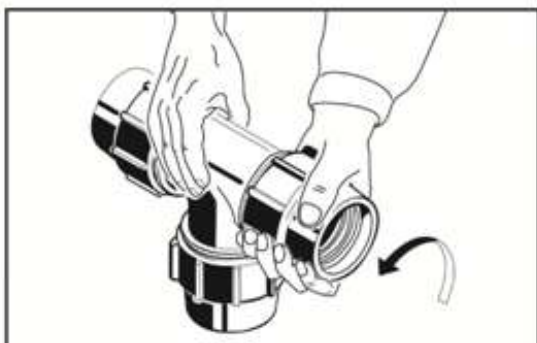
Step1: Unscrew the nut, remove the compression ring and o-ring without removing the integral component locked inside the nut.
