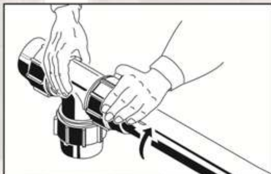
Step 4: Slide the nut over the grip ring on the body and tighten it.
