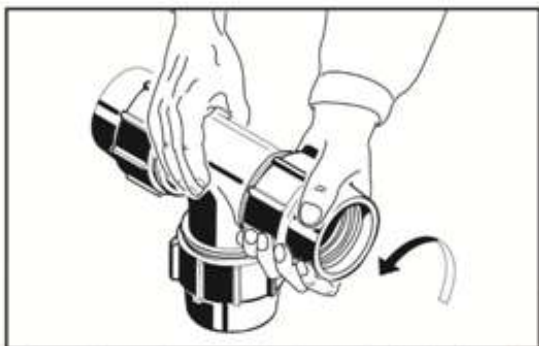
Step1: Unscrew the nut and the grip ring. Put the pipe through the nut and the grip ring with the conic part facing the nut.
