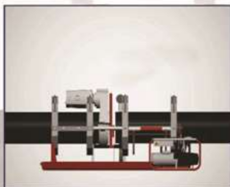
Step3: Facing unit is moved into position. Switch on the facing unit and bring the clamp slowly together.
